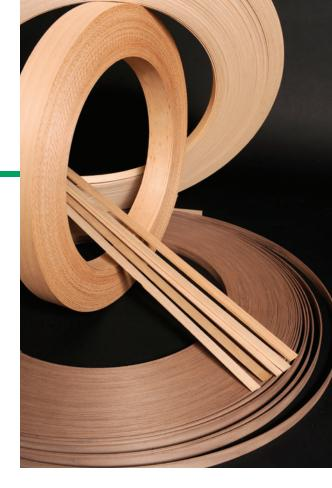
Thick veneer coils offer many advantages and efficiencies over solid strips. Coils provide high machine throughput, minimize waste, and reduce edgebanding inventory requirements. They also provide a product that will not warp or twist and has consistent thickness and width. Only natural wood inner plies and A-grade face veneer are used; reconstituted veneers are not substituted for inner plies, unless specified by the customer.
